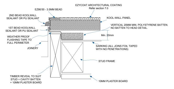
\*NOTE: WHEN INSTALLING KOOL-WALL PANELS TO WINDOW AND DOORS MAINTAIN A GAP OF 3 TO 4MM AROUND THE PENETRATIONS IN ORDER TO ACCOMODATE THE REQUIRED KOOL-WALL SEALANTS.
